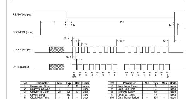
Synchronous Timing Diagram (Note: Asynchronous mode timing is per RS-232. To use RS-232 requires the Maxim MA232 interface circuit for proper voltage level compatibility.)
